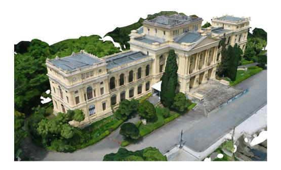
Figure 19 – Electronic model of the building-monument of Museu Paulista, generated by drone aerial survey.
