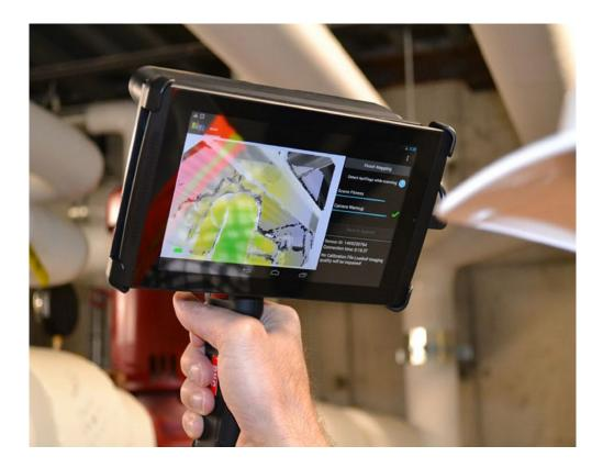
Figure 6 – Trimble DPI-8 handheld scanner. Photograph by the authors.
