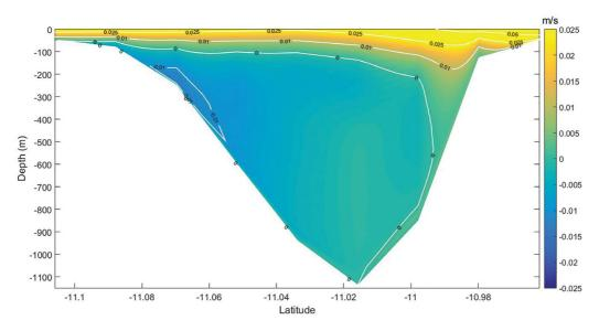
Figure 11. Velocity perpendicular to the vertical section of the canyon (positive values indicate subsidence, negative values indicate downward motion) for southeast simulation.
