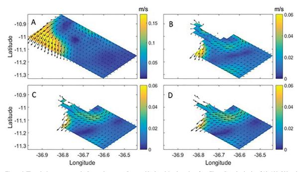
Figure 6. The velocity vectors near the Japaratuba canyon (between North and South sections from Figure 2) at the depths of 10, 100, 200 and 300 meters (panels A, B, C and D, respectively) for Northeast Wind simulation and homogeneous temperature and salinity fields (experiment C1).
