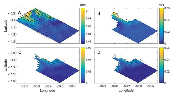
Figure 10. Circulation around Japaratuba canyon at depths (between North and South sections from Figure 2) 10, 100, 200 and 300 meters (panels A, B, C and D, respectively), for Southeast winds simulation.
