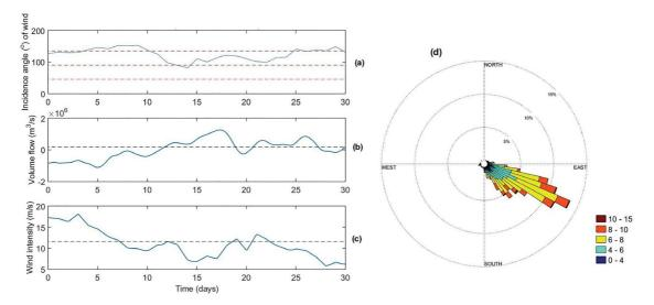
Figure 17. Incidence angle of average wind (a), Volume flow in the canyon section (b), intensity of average wind (c), and the wind rose (d), in the simulation for September 2014 (experiment R3).
