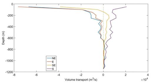
Figure 12. Volume flow perpendicular to the section of Japaratuba canyon (positive values indicate subsidence, negative values indicate upward motion), for NE, E, SE and S winds simulations and homogeneous temperature and salinity fields (experiments C1 to C4), integrated every 50m.
