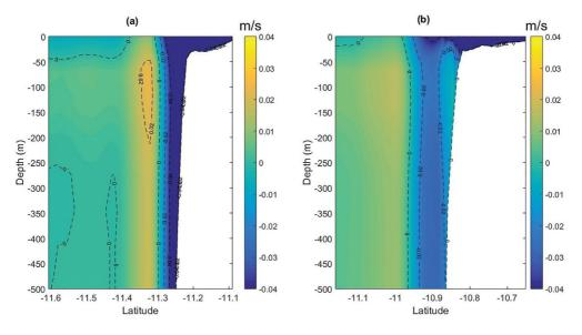
Figure 5. Velocity parallel to the coast at the South (panel A) and the North (panel B) of the Japaratuba canyon (North and South sections from Figure 2), for simulations with NE winds. Positive velocity going to NE and negative velocity going to SW
