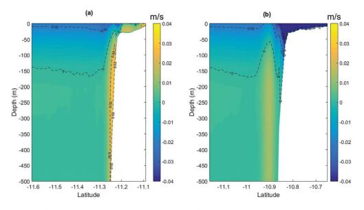
Figure 9. Velocity parallel to the South (panel A) and to the North (panel B) of the Japaratuba canyon (North and South sections from Figure 2), for simulations with SE winds. Positive velocity going to NE and negative velocity going to SW.
