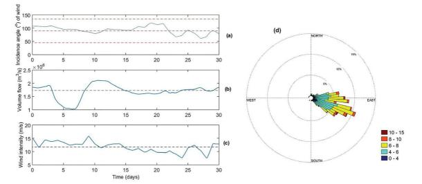
Figure 16. Incidence angle of average wind (a), Volume flow in the canyon section (b), intensity of average wind (c), and the wind rose (d), in the simulation for July 2014 (experiment R2).
