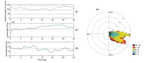
Figure 15. Incidence angle of average wind (a), Volume flow in the canyon section (b), intensity of average wind (c), and the wind rose (d), in the simulation for March 2014 (experiment R1).
