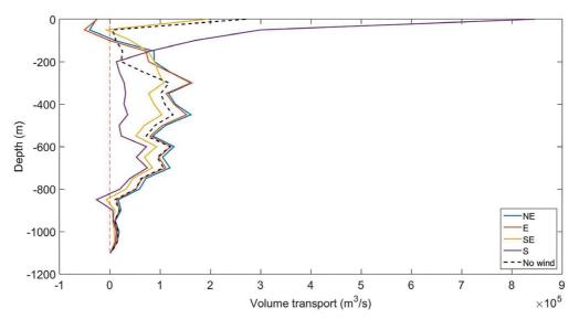
Figure 14. Volume flow perpendicular to the section of Japaratuba canyon (positive values indicate subsidence, negative values indicate upward motion), for NE, E, SE and S winds simulations (experiments C5 to C8) and without wind (experiment NW) with stratified temperature and salinity fields, integrated every 50 m.
