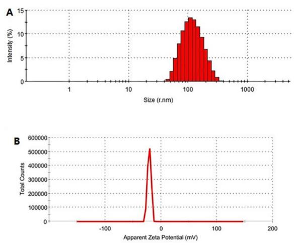
FIGURE 1 - Particle size and zeta potential of 2-ME-PSL.
