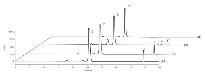
**FIGURE 2** – Representative SE–LC chromatograms showing peak  $1 = rhIFN\beta-1b$ ; peak 2 = human serum albumin; peaks 3 and 4 = high–molecular–weight substances. (a) Biological reference substance of rhIFN $\beta$ –1b. (b) Sample of biopharmaceutical formulation, untreated and after: (c) neutral hydrolysis; (d) placebo.
