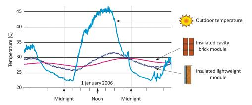
Figure 4. Thermal performance of cavity brick versus lightweight housing test modules.
