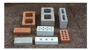
Figure 1. Typical Australian masonry units.
