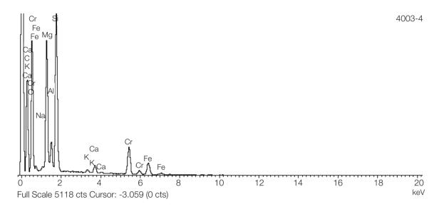
**Figure 15.** Energy dispersive x-ray spectrometerspectra of sample II-B: the peak of silicon stands out, followed by the iron, chromium, calcium, aluminum and potassium peaks.
