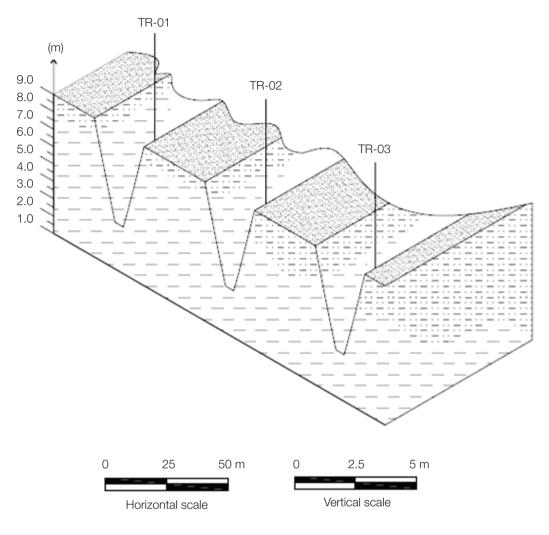
Figure 5. Profile of waste sample collection – Group B.
