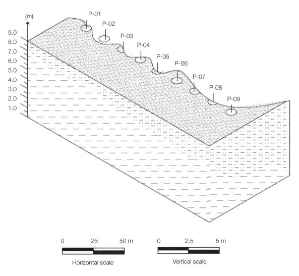
Figure 2. Profile of waste sample collection – Group A.
