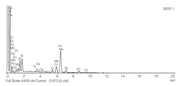
**Figure 11.** Energy dispersive x-ray spectrometer spectra of sample IV-A: the peak of calcium stands out, following by the iron, manganese, chromium and zinc peaks.
