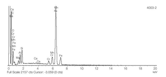
**Figure 14.** Energy dispersive x-ray spectrometer spectra of sample II-B: the peak of calcium stands out, followed by the iron, manganese and chromium peaks.
