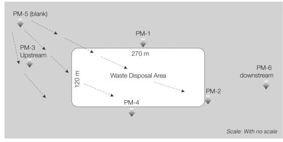
Figure 9. Location of monitoring wells and flow of groundwater.
