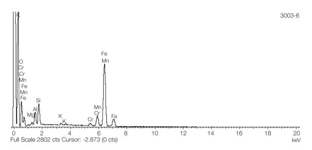
**Figure 12.** Energy dispersive x-ray spectrometer spectra of sample IV-A: the peak of K stands out, following by the iron, manganese, silicon and chromium peaks.
