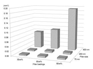
Figure 4- The correlation of the wear volumes between the two factors after 40,000 cycles
