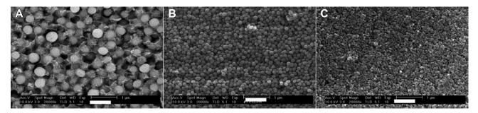
(A) Mean filler diameter of 400 nm; (B) Mean filler diameter of 200 nm; (C) Mean filler diameter of 70 nm
