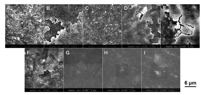
(A) Group 1; (B) Group 2; (C) Group 3; (D) Group 4; (E) Group 5; (F) Group 6; (G) Group 7; (H) Group 8; (I) Group 9 (A), (B) and (C), Individual filler particles can be detected on the worn surface.; (D), (E) and (F), a defect with cracks was observed on the specimens.; (G), (H) and (I), the worn surfaces on the specimens were extremely homogeneous
