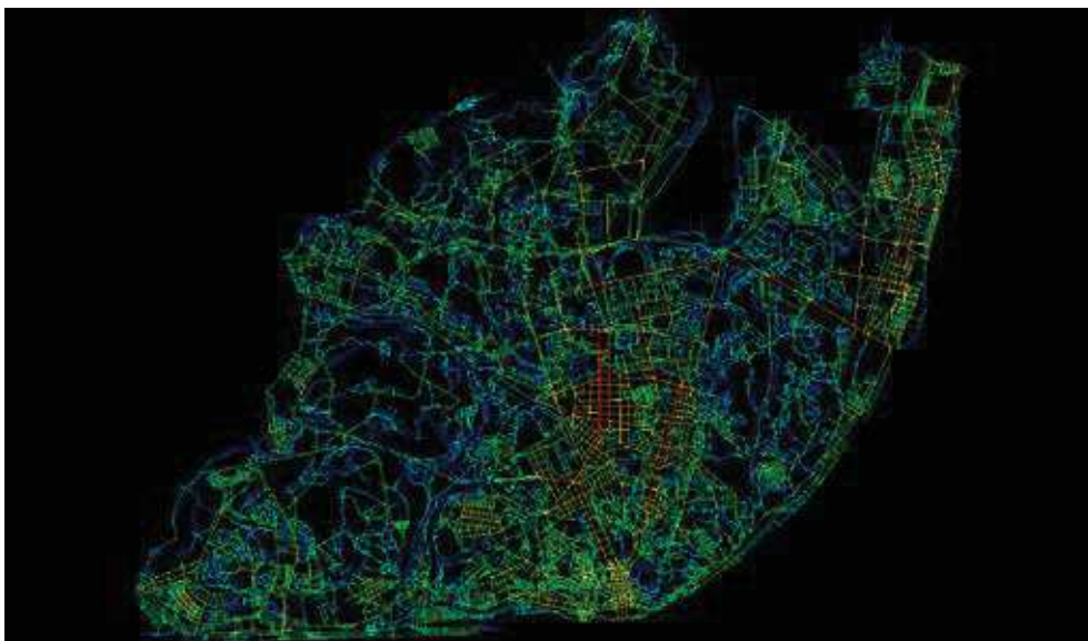
Figure 1b Local integration of the streets. Map showing the local integration of Lisbon's streets system. The warmer colours, closer to red, represent parts of the city with higher values of local integration. The cooler colours, towards dark blue, represent parts of the city with lower values. Source: João Pinelo Silva e Teresa Heitor, 2013.
