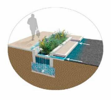
Figure 15: Three-dimensional model of the operation of a rain garden on the sidewalk Source: Adapted from Philadelphia Water Department, 2014.
