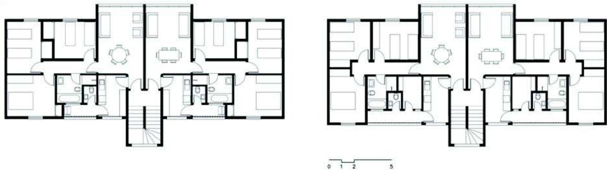
Fig. 10: Floor plan of 85 m<sup>2</sup> and 89 m<sup>2</sup> apartments
