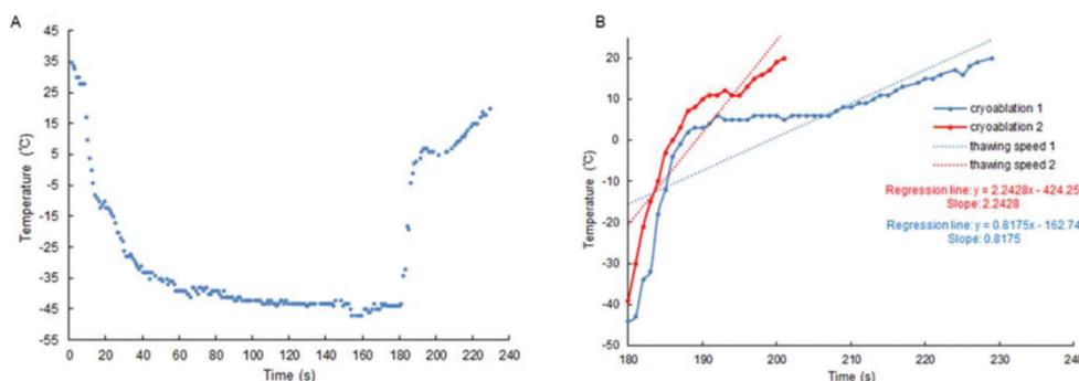
**Figure 1** - Examples of cryoablation curves and their fitted regression line A, Example of a complete cryoablation curve. B, Examples of a portion of the cryoablation curve (the time frame from the first value > -50°C, with 60s duration) and their fitted regression line.
