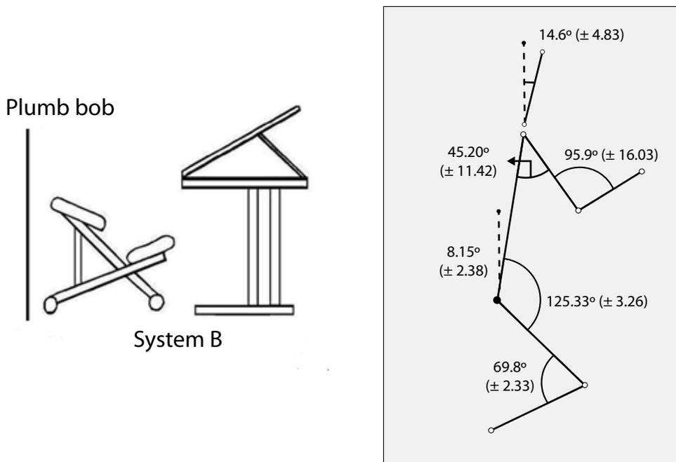
Figure 2. Posture induced by the experimental chair-desk system (system B)
