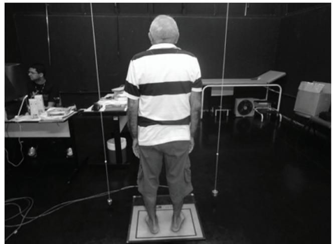
Figure 1. Acquisition of stabilometric data
