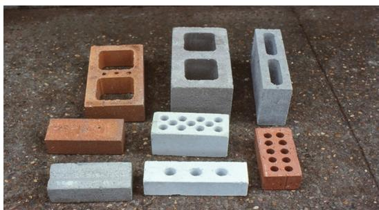
Figure 1. Typical Australian masonry units.
