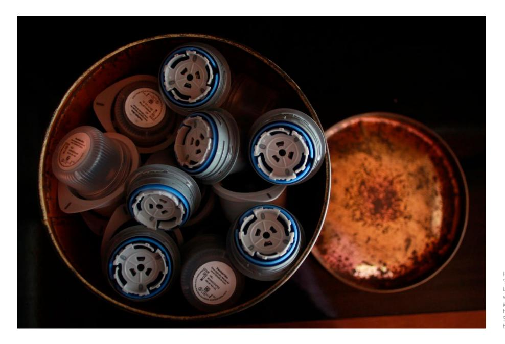
FIGURE 10 Sensor applicators that allow the verification of blood glucose without finger piercing. Source: https:// bit.ly/2xoKOSE.
