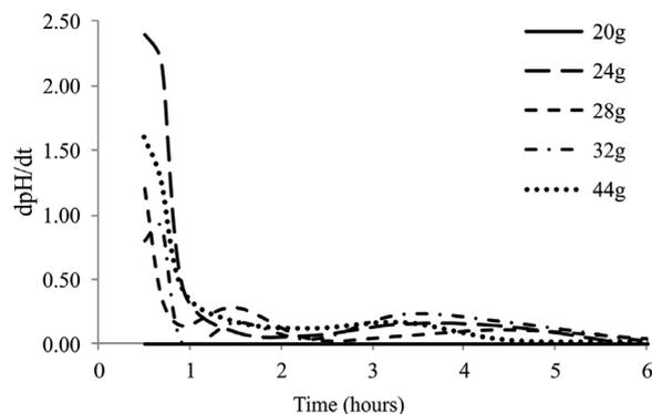
**Figure 3.** First derivative of the pH-value as a function of time (dpH/dt) in the experiment using acidic effluent and marble waste.
