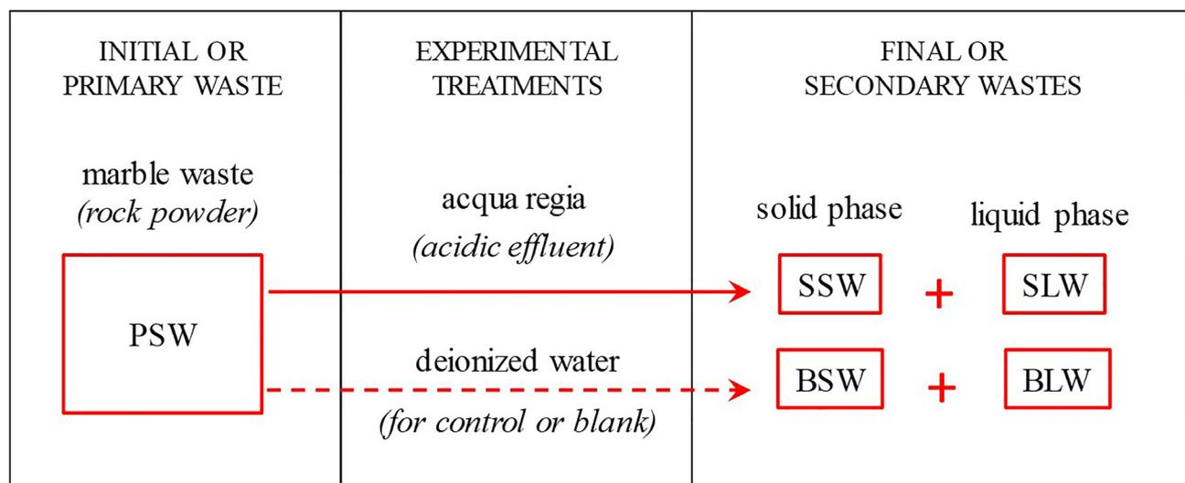
**Figure 1.** Outline of the experimental strategy adopted in this work (PSW = primary solid waste or marble dust; SSW = secondary solid waste; SLW = secondary liquid waste; BSW = solid phase of the analytical blank, and BLW = liquid phase of the analytical blank).
