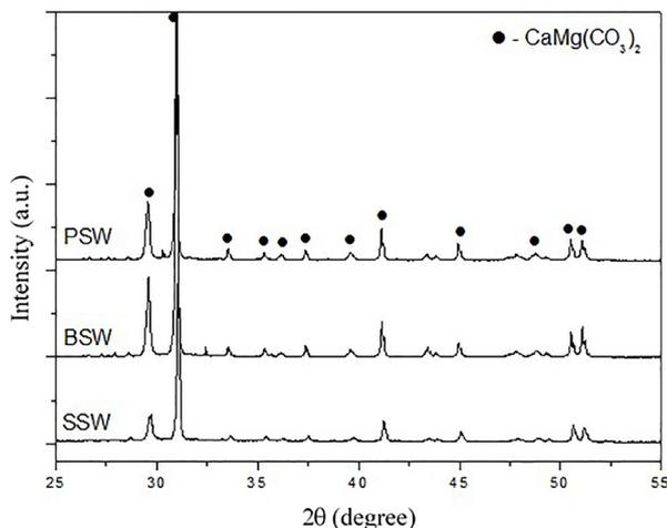
**Figure 7.** Mineralogical composition of the marble dust used in the experiment (PSW), the solid fraction of the analytical blank (BSW), and the solid phase obtained after treatment of the acidic solution (SSW).
