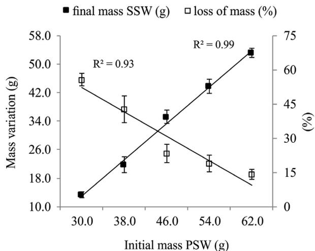
**Figure 6.** Mass loss of the secondary solid waste (SSW) relative to the mass of primary solid waste (PSW) used to attenuate the acid effluent.
