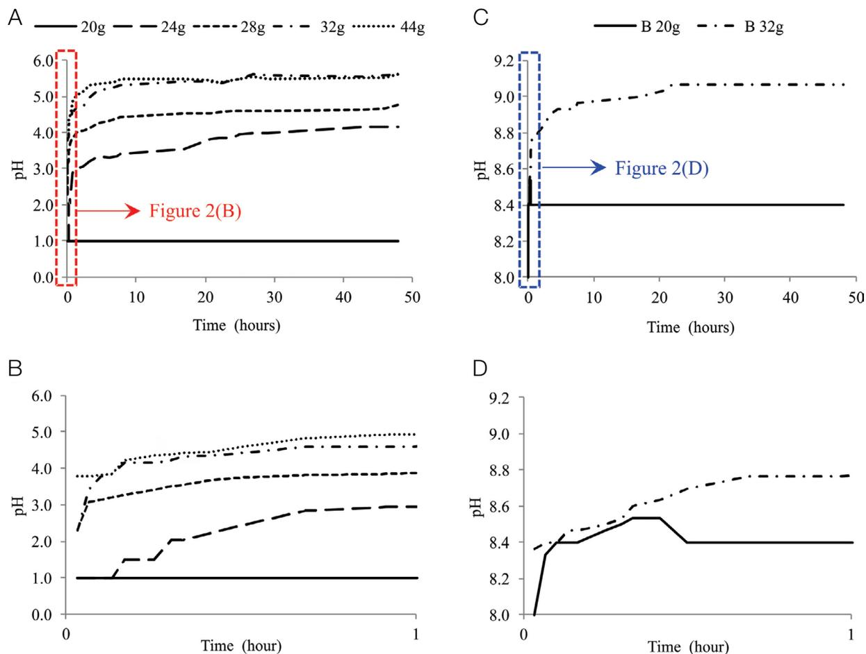
**Figure 2.** (A) Variation in pH-value of the acid effluent with increasing quantities of marble waste and (B) detail of the red dashed part, considering the first one hour of the experiment. (C) Variation in pH-value of the analytical blank using deionized water with marble waste and (D) detail of blue dashed part showing the blank experiment in the first one hour.
