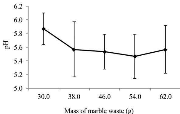
**Figure 4.** pH values measured in the SLW (Secondary Liquid Waste) resulting from each treatment of the acidic effluent with marble waste.
