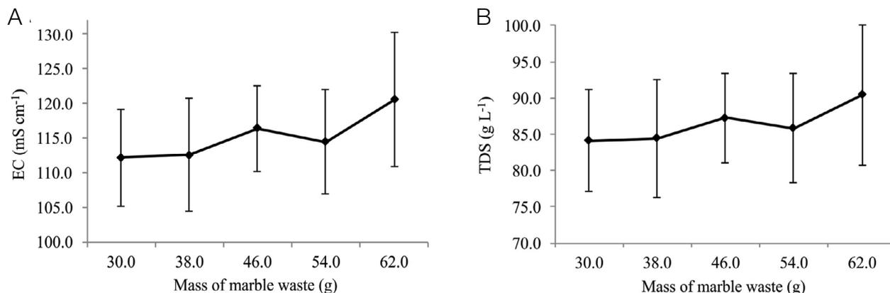
**Figure 5.** (A) Electrical conductivity (EC) and (B) estimated total dissolved solids (TDS) in the SLW obtained after 5 hours of reaction.
