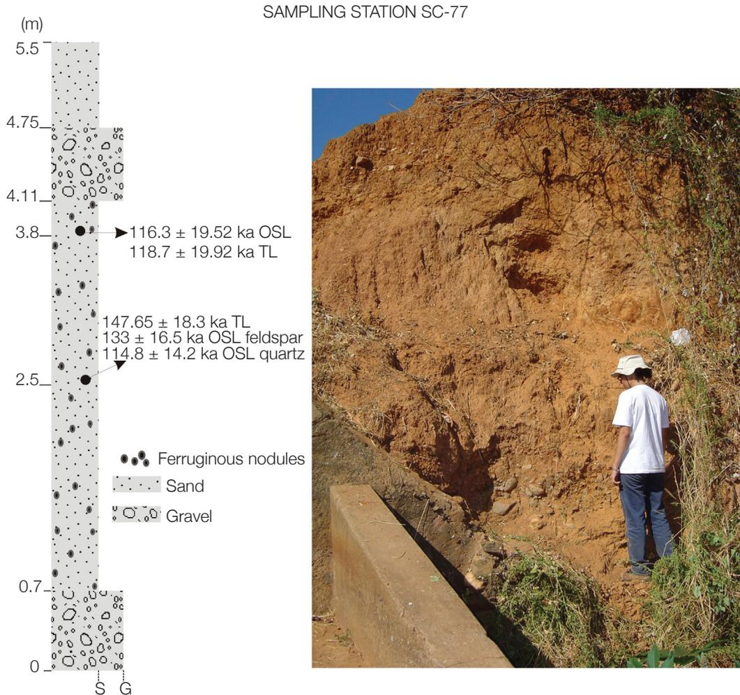
**Figure 9.** Sampling station SC-77, it is possible to see a 5.5 m thick alluvial deposit composed of alternating gravel and sand beds deposited by the Piauí River.
