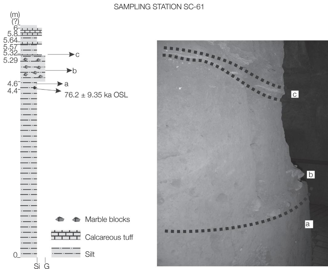
**Figure 7.** Columnar section of the sampling station SC-61 (Toca de Cima dos Pilão cave), which is a cave filled by at least 6 m thick sediments. At the top, there is an alternated sequence of calcareous tuff and mud. The photo shows sandy mud (a) and gravelly (b) and calcareous tuff (c) deposits.
