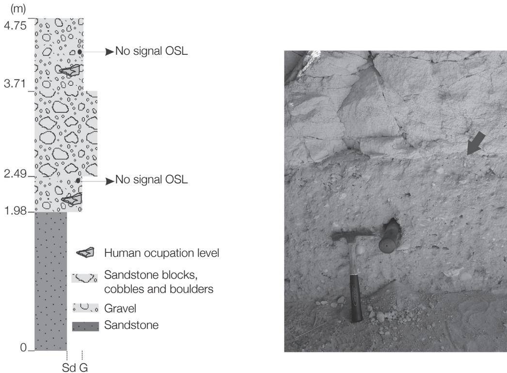
**Figure 6.** Sampling station SC-49 (Sítio do Meio rock shelter) in the Southern Structural Staircases colluvial deposit presents two gravel beds and a bed of fallen rock. This photograph shows the contact between the first gravel bed and a bed of fallen rock.
