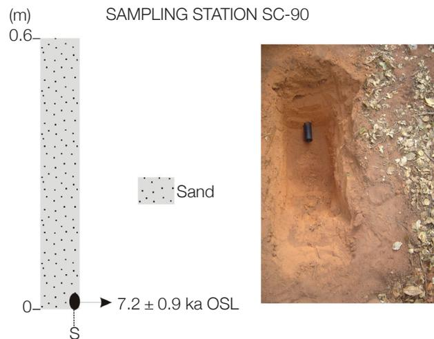
**Figure 3.** Sampling station SC-90 composed of sandy eluvial-colluvial deposits. Observe the PVC sampling tube for luminescence dating.
