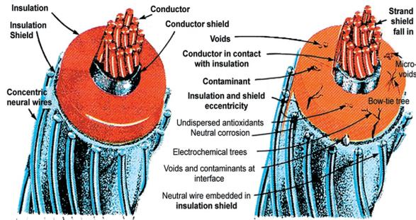
**FIGURE 17-** The term “water tree” was originated from the tree-like deterioration patterns that were found within the polyethylene insulation of underground electrical cables
