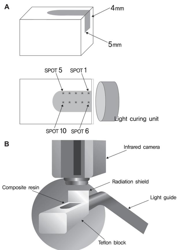
**Figure 1-** (A) Schematic diagram of the temperature measurement spots from spot 1 to 10. (B) Schematic diagram of infrared thermographic measurement of temperature change in the composite resin during photopolymerization. The infrared thermographic camera was located above the composite resin in a Teflon block. A radiation shield was used to limit the radiation of the light guide only to the proximal surface of the composite resin
