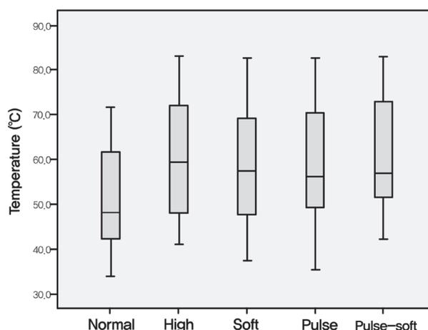
**Figure 2-** Mean peak polymerization temperature ( $^\circ\text{C}$ ) of composite resin specimens at the selected spots according to the light curing modes of light emitting diode light curing unit ( $p > 0.05$ )
