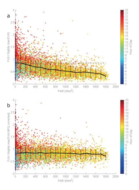
**Figure 6.** The ratio maximum nighttime  $F_{chl}$  to  $F_{chl}$  for non-quenching (a) and quenching-corrected (b) measurements as function of incident PAR over SiMCosta SC01. The dashed line represents the mean value of the ratio at nighttime when solar radiation is null. Median and standard deviation of  $F_{chl}$  values are shown by solid black line and error bars, respectively, at PAR intervals of 100 W m<sup>-2</sup>. The colors are associated with the hour (GMT time) of the day.
