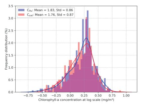
**Figure 7.** Distribution of 506 paired data which were considered valid for the match-up procedure between  $C_{nu}$  (blue color) and  $C_{sat}$  (orange color). The mean and standard deviation values for  $C_{nu}$  and  $C_{sat}$  were 1.83±0.86 and 1.76±0.87 mg m<sup>-3</sup>, respectively.
