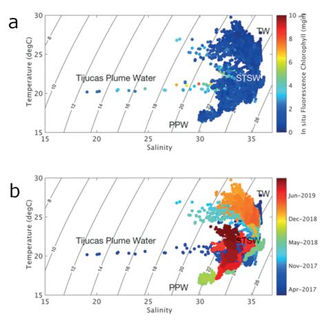
Figure 4. TS-fluorescence (a) and TS-time (b) diagrams. TW, STSW and PPW stand for Tropical Water, Subtropical Shelf Waters and La Plata Plume Water. The effect of the plume of Tijucas river on the local thermohaline properties is also shown.
