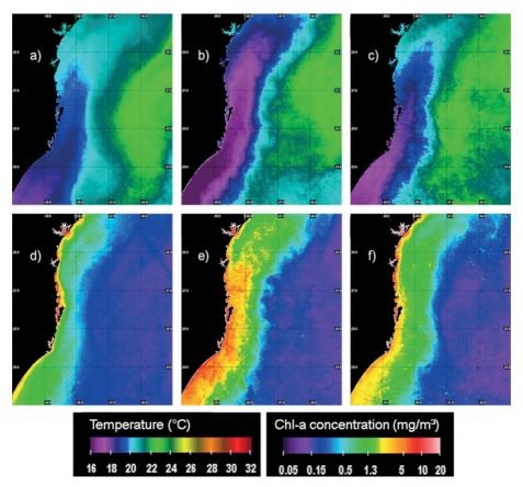
Figure 8. Monthly mean MODIS/VIIRS composite of daily sea surface temperature (SST) in July 2017 (a), July 2018 (b) and July 2019 (c) and monthly mean MODIS/VIIRS composite of daily chlorophyll-a surface concentration in July 2017 (d), July 2018 (e) and July 2019 (f). The SST images were derived from the NLSST algorithm and represent a composition of daily MODIS-Aqua, MODIS-Terra, VIIRS-JPSS and VIIRS-NOAA20.
