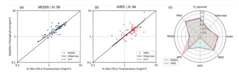
**Figure 10.** Comparisons between  $C_{flu}$  and  $C_{sat}$  for sensor MODIS and VIIRS at logarithm (a and b) scales using straylight flags (at least 5 valid pixels). The star plots of the metrics used to compare  $C_{flu}$  and  $C_{sat}$  at logarithm (c) scales are also shown.
