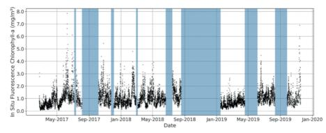
Figure 3. Temporal series of hourly Fchl data (black dots) approved by the SiMCosta data quality control system. The gaps (blue stripes) correspond to 27% of the entire dataset, and usually they are associated with maintenance of sensors and/or electrical failure of the power system of the SiMCosta-SC01 buoy.
