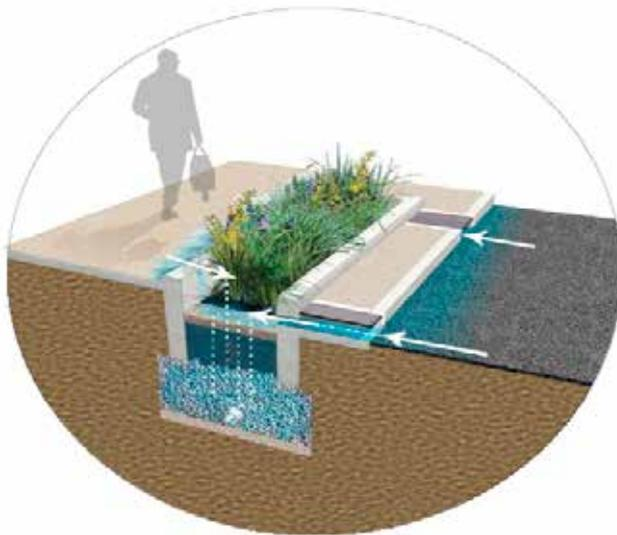
Figure 15: Three-dimensional model of the operation of a rain garden on the sidewalk
