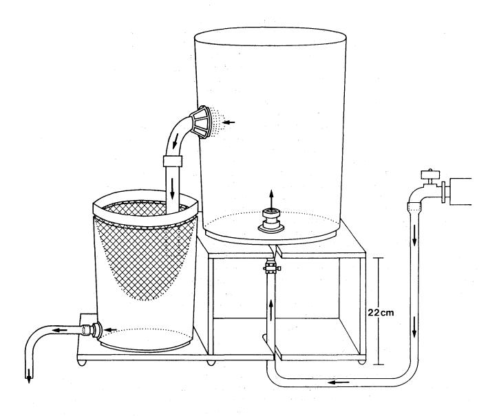
Fig. 1. Diagram of the elutriator. Larger cylinder with 37 x 29 cm. Smaller cylinder with 11 x 19 cm, conic sieve of 270  $\mu$  nylon screen.
