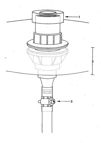
Fig. 2. Detail of the terminal part of the tube which transport the incoming water to wash the sediment. 1: a 270  $\mu$  sieve with 3.5 cm in diameter at the end of the PVC tube; 2: a system of PVC nuts to enlarge tube diameter; 3. steel clamp.
