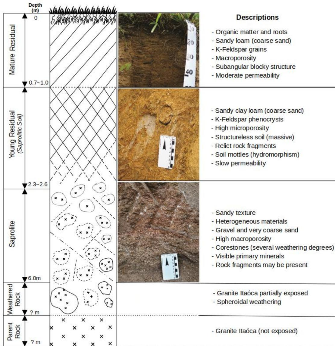
**Figure 3:** Typical weathering profile in Itaóca granite (Brazil). The profile shows clear differences in soil color, texture, and macrostructure with depth. Three zones were defined: mature residual, young residual, and saprolite.
