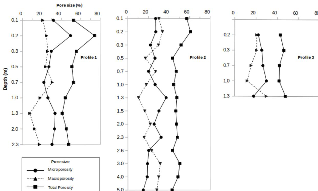
**Figure 5:** Soil porosity distribution in weathering granitic profiles 1, 2, and 3. Changes in microporosity and macroporosity distribution can be linked to clay content. Total porosity is not affected by clay content.
