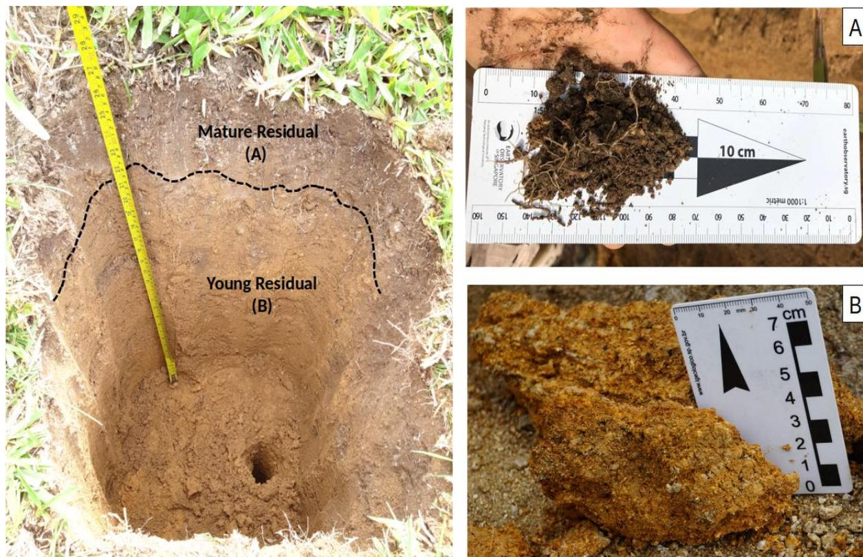
**Figure 4:** Contact between soil layers with potential rupture zone (black dotted line). Clear differences in soil color and macrostructure (A) Mature residual soil presents a crumb structure and dark color at upper surface and (B) Young residual (Saprolitic soil) presents a massive structure and a light color material.
