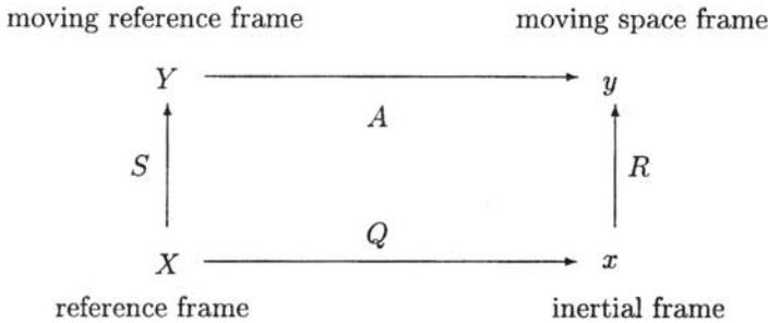
Figure 1: Coordinate systems for an affine rigid body.
