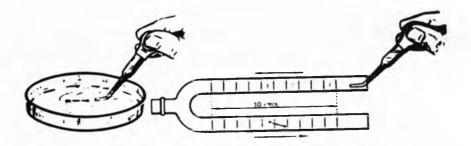
Fig. 2 — The technique for measuring the unidirectional mobility of the isolated tentacle. The graduated capillaries of a standard Warburg manometer were filled with the proper medium previously to the introduction of the tentacle into the capillary tubes. The tentacles were first sucked up into a small pipette and then introduced into the capillary tubes. The mobility was then measured as the time taken by the isolated tentacle to move through a fixed distance of 100 mm.
