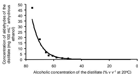
Figure 3 – Volatilization kinetics of aldehydes, in acetic aldehyde, during the first distillation.
