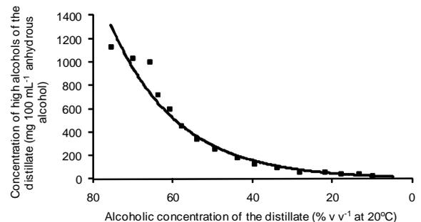
Figure 7 – Volatilization kinetics of high alcohols (propyl + isobutyl + isoamyls) during the first distillation.
